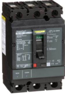
Circuit breaker, PowerPact H, 100A, 3 pole, 600VAC, 18kA, lugs, thermal magnetic, 80%
