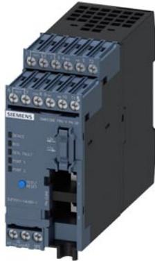
Basic unit SIMOCODE pro V PN GP Ethernet/PROFINET IO, PN system redundancy, OPC UA server, Web server, transmission rate 100 Mbps, 2 x bus connection via RJ45, 4 I/3 Q freely parameterizable, Us: 110...240 V AC/DC, input for thermistor connection Monostable relay outputs, expandable by 1 extension module(DM, TM, EM)
